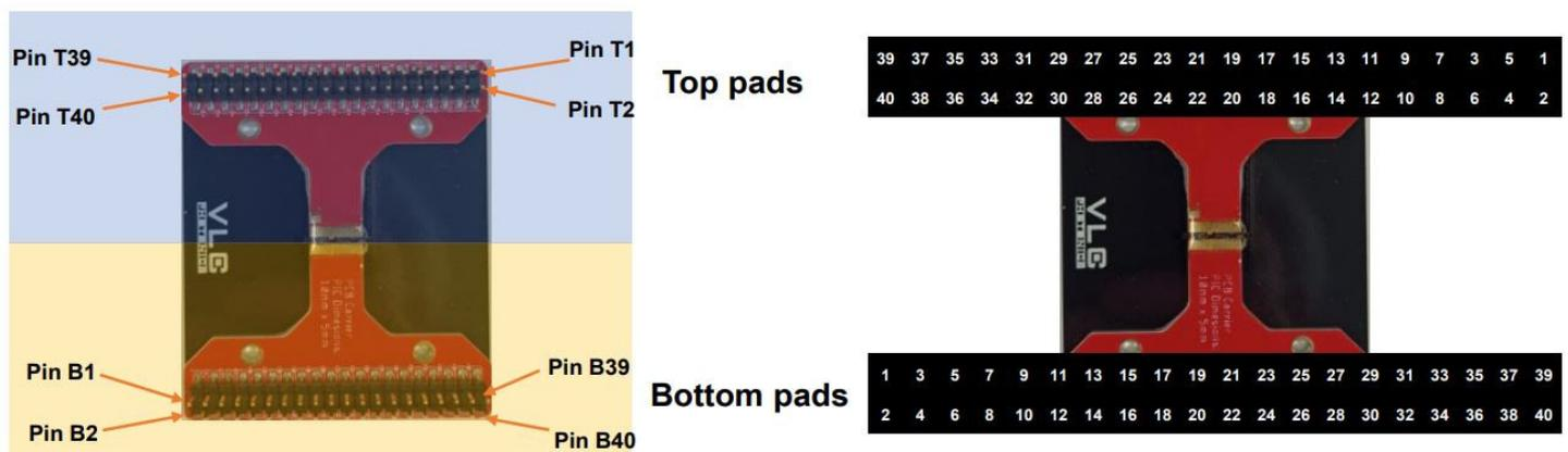
FIGURE 60: PACKAGING OF THE CHIP SHOWING THE ELECTRICAL CONNECTIONS
